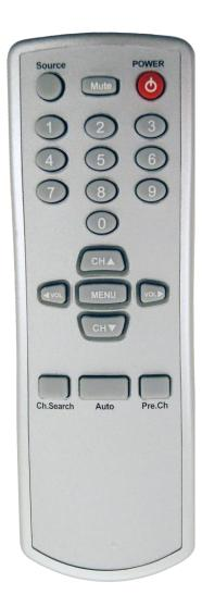
The remote control included with the FD102CV contains the same functionality available on the display buttons, to include power, source, menu, and directional arrows.
