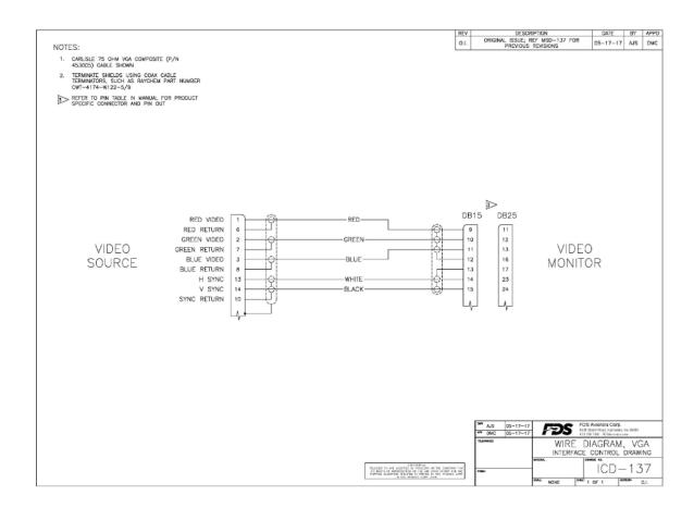
The individual wires should be extended with 6" 22awg wires using an environmental splice for the red & green wires, and Raychem caps for the blue, white, and black wires.
