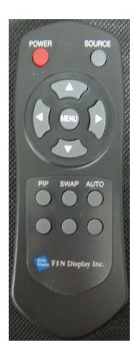
The remote control included with the FD102CV contains the same functionality available on the display buttons, to include power, source, menu, and directional arrows.
